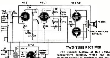
regenerative receiver, which has an amazing amount of sensitivity and output volume, is in the r.f. tuning section. Instead of the usual high-impedance an-
